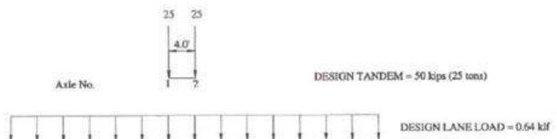
HL-93 Design Tandem with Lane Load
